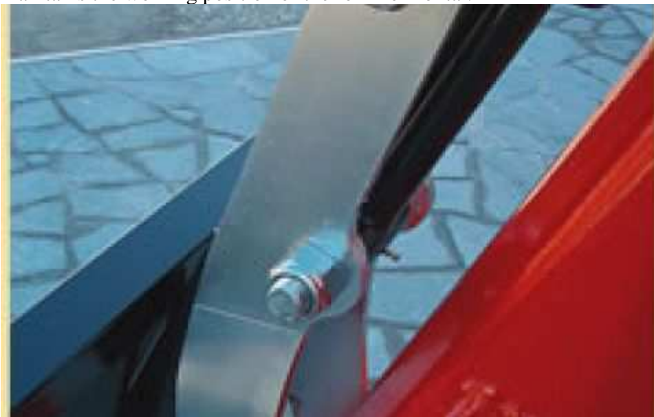
1) Parallelogram which maintains the working position of the fork horizontal.
