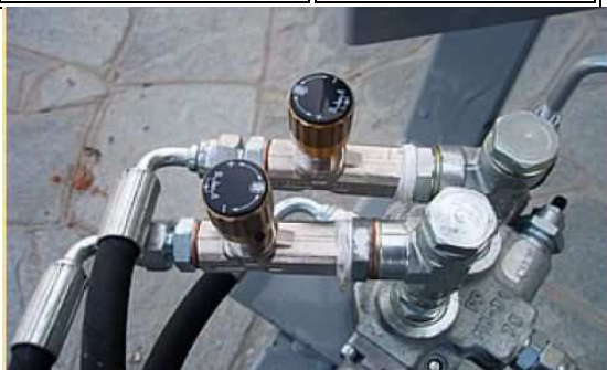
A detail of the forward-reverse drive flow regulator
