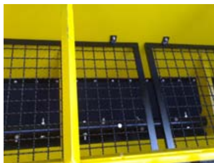
Inner safety net to avoid contact with parts in action.
