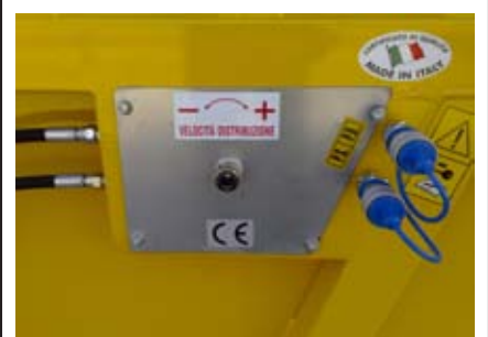
Capacity load regulator to weight compensation.
