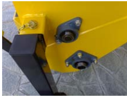
Lateral bearings subject to lubrication each 30 hours of work.
