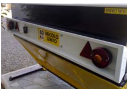
Back lighting used during road transportation
