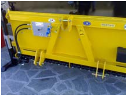
Connection in 3 points for agricultural tractor (if request available on operator machines).
