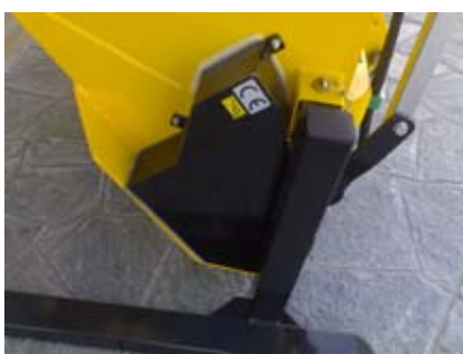
External driving chain protect with case to avoid contact with moving gears.
