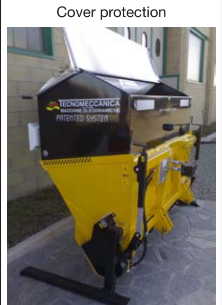
Lateral support feet (to be removed during work).
